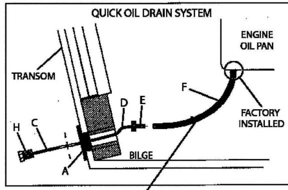
5. Pull the oil drain plug (E), and the oil drain hose (F) through the garboard drain.
