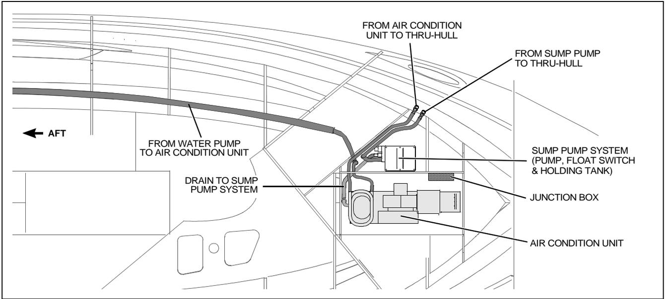
***Air Conditioning Duct Routing***
