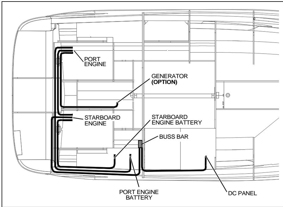
**Negative Battery Cable Harness (Diesel Option)**
