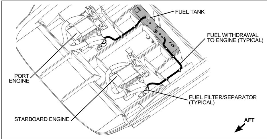
**Diesel Fuel System Routing (Option)**
