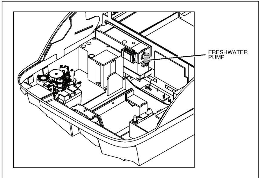
**Freshwater Pump Switch:** Located just forward of the galley sink.
