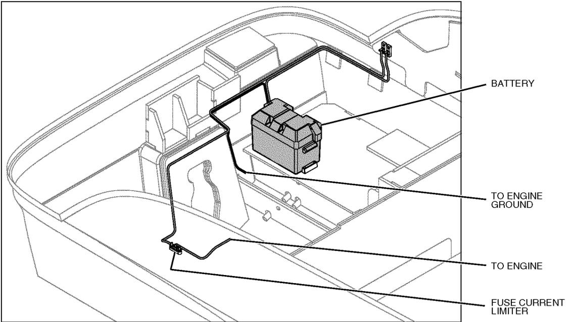
BATTERY CABLE ROUTINGS (IF EQUIPPED WITH DUAL BATTERY)
