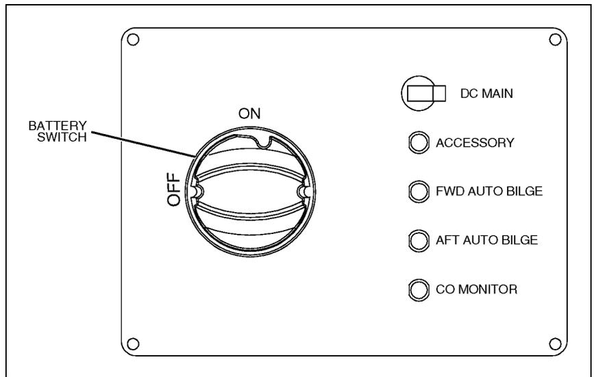
**Battery Switch (If Equipped with Two Batteries)**
