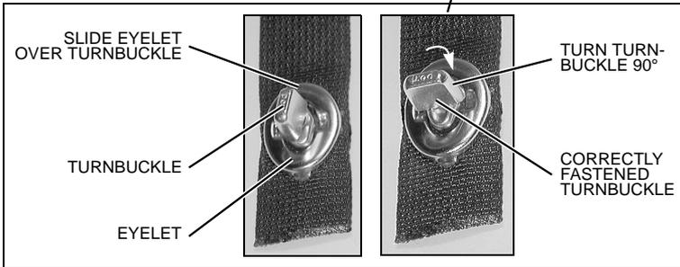
**Step - 4b for 1950BT:** As shown above, attach the safety straps to the turnbuckles on the on the aft wall of the cockpit.
