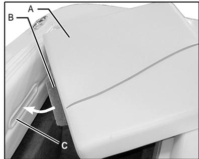
**Step - 3:** Press down firmly on the inboard side of each jump seat until they rest firmly on the motorbox ledges.
