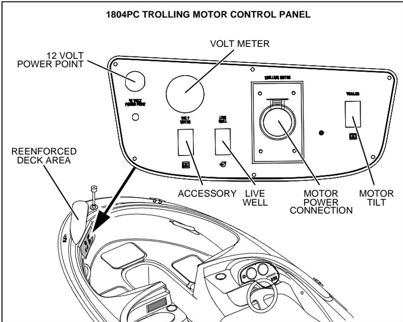
The trolling motor system can be used safely with both a 12V or a 24V motor. However, the voltage gauge will only register with a 24V motor.
