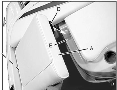
**Step - 3:** Press down firmly on each jump seat until they rest firmly on the cockpit and motor box ledges.
