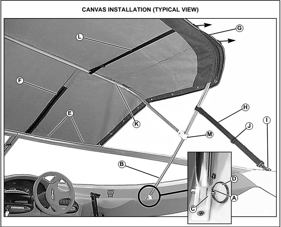
1. Insert eye ends (A) of main bow (B) into deck hinges (C) and secure with pins (D).
