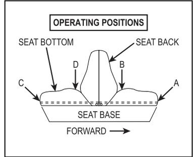
6. Lock the aft seat into position by pushing down at point (C).
