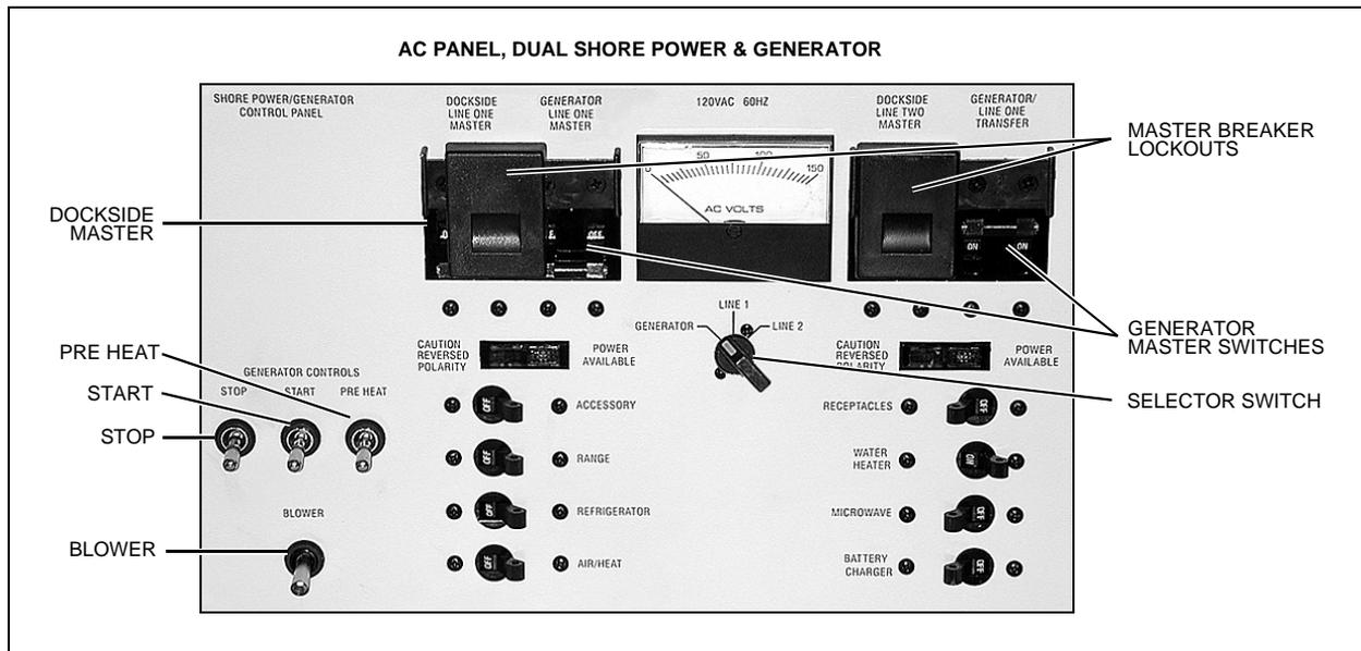
1. Run the bilge blowers for a minimum of four minutes *before* starting the generator.
