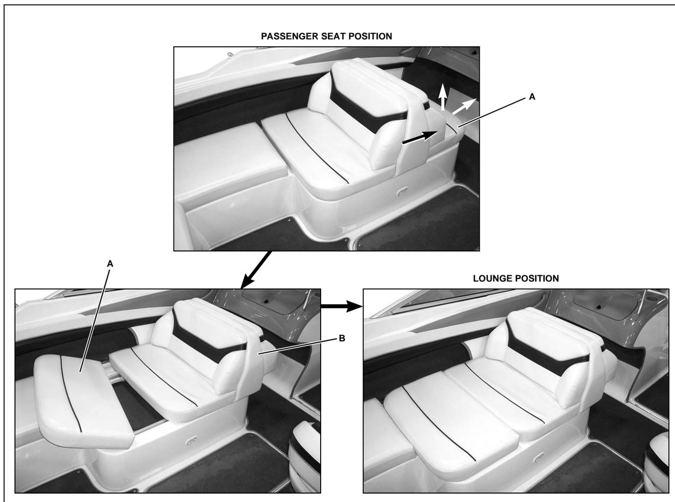
1. Remove the forward seat bottom (A) by lifting and pulling the forward edge.
