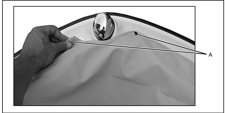
3. On the starboard side, only snap the forward half of the bow cover to the deck.
