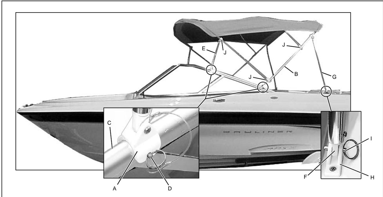
1. Slide the swivel ends (A) of the main bow (B) over the aft pre-drilled holes in the windshield frames (C) and insert the pins (D).
