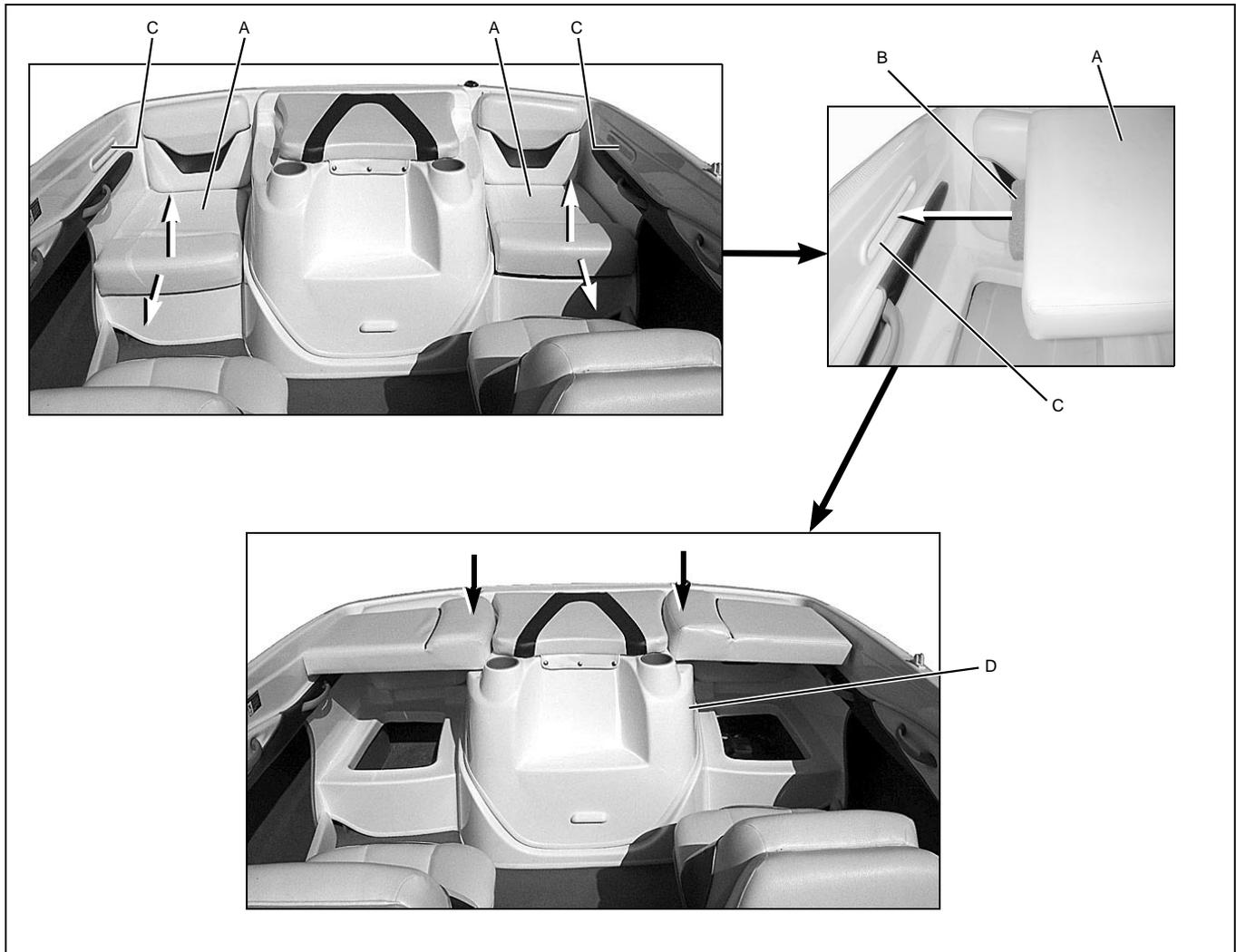
1. Remove the jump seats (A) by lifting and pulling on their forward edges.
