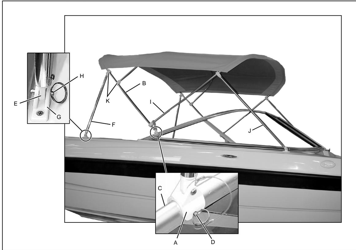
1. Slide the swivel ends (A) of the main bow (B) over the pre-drilled holes in the windshield frames (C) and insert the pins (D).
