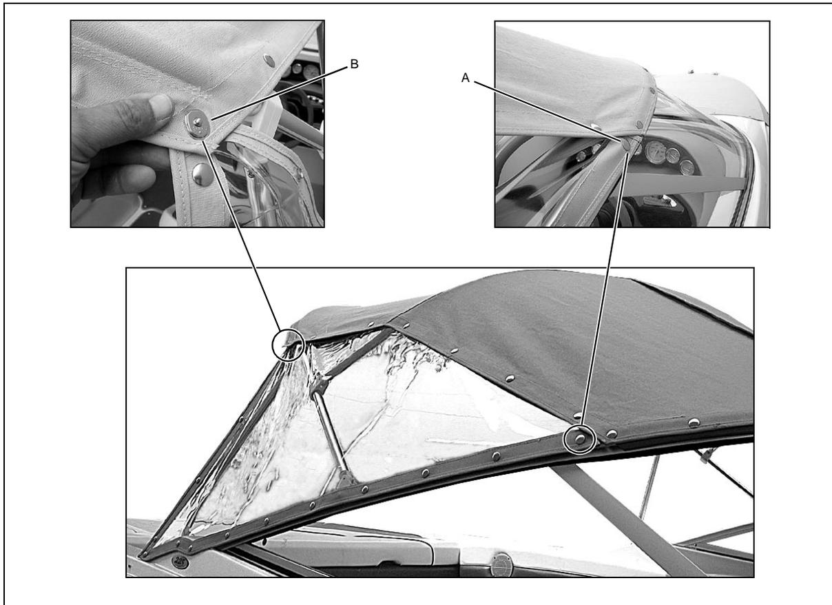
1. Snap the forward corner of the side curtain (A) to the windshield frame.
